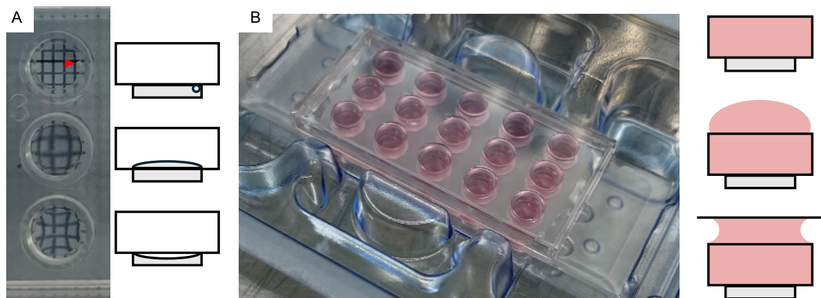
Figure 1. Preparing the ibidi slide. A) Examine if the Matrigel layer is flat and free of bubbles (red arrow) by placing the slide on top of a fine grid and checking for any warping of the lines. B) After seeding the cells, gently place a drop of medium on top of each full well to create a dome and ensure contact between the medium and the lid.
